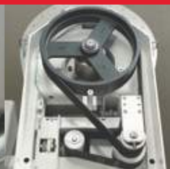
Mechanical reduction with pulleys and belts
