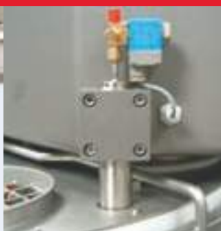
CO 2 injection valve
